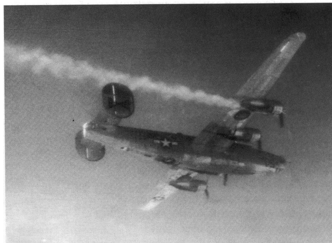
A 461st Bomb Group B-24 drops out of formation with #4 engine on fire after leaving the combat zone. Note: the lower ball turret is retracted. This indicates that the gunner has exited the turret
