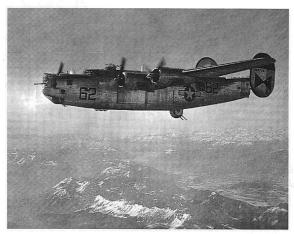
No #62 with the Sperry Ball Turret down: Used by both the B-17 (not retractable) and the B-24, it was cramped and cold and suffered the indignity of being in line with the forward relief tubes.
