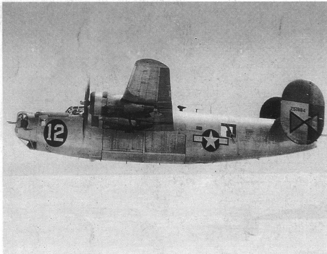
42-51884 a Ford built B-24J, 824 sq. shows a white number on a round black background on the nose only. The round background was used exclusively by the 484th Bomb Group later in the war for improved recognition from a longer distance. The left rudder has been replaced as the color is slightly lighter. Note the waist windows are covered with plexiglass. This aircraft was also equipped with anti aircraft radar jamming electronics.
