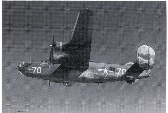
42-52683 A Ford built B24H "The Uninvited" shows a typical white on olive color scheme.. The waist window displays a local modification. Note the de-icer boots have been removed.
