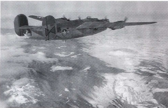
42-51851 Ford Built B-24J Shows the Consolidated tail turret, Note: the inside of the left rudder is painted red.
