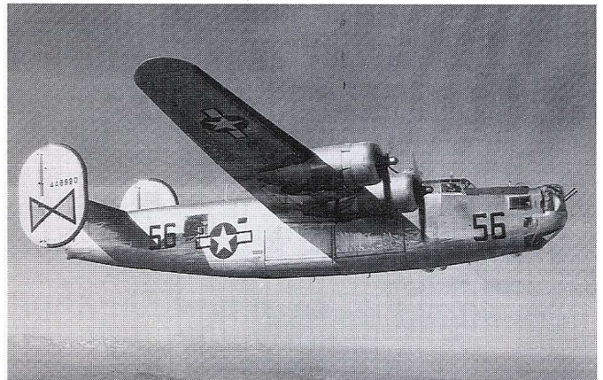
44-49890, A Ford Built B-24L, 826 squadron. De-icer boots still in place and equipped with three flak suppression radio transmitters
