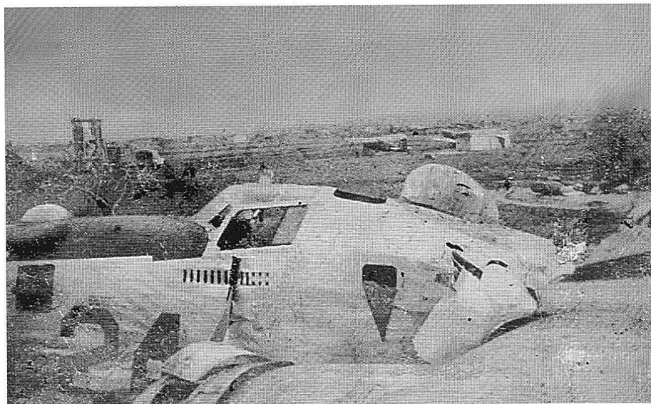
No 3 propeller sliced into the skin of the plane and into the Captain's seat.
