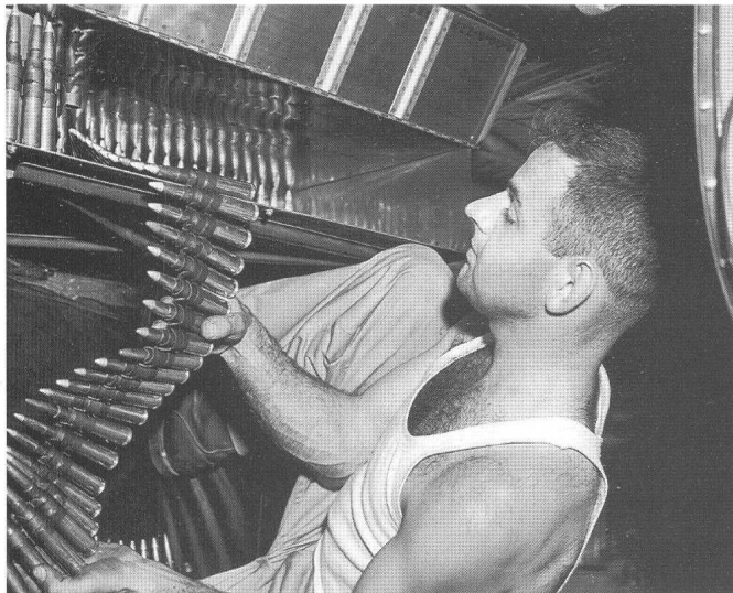
Loading waist gun ammunition can, Every fifth round was a tracer shell as indicated by the color of the bullet tip.
