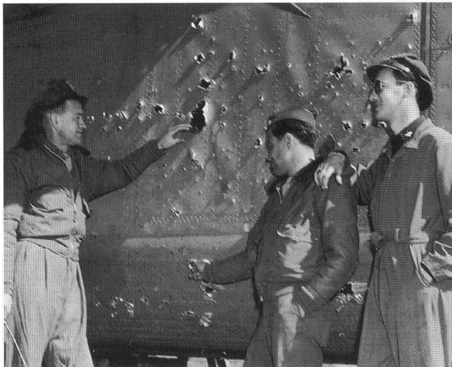
Crewmen examine bomb damage on a 461st Bomb Group B-24. An anti aircraft shell entered the bomb bay from below exploding on the opposite side.
