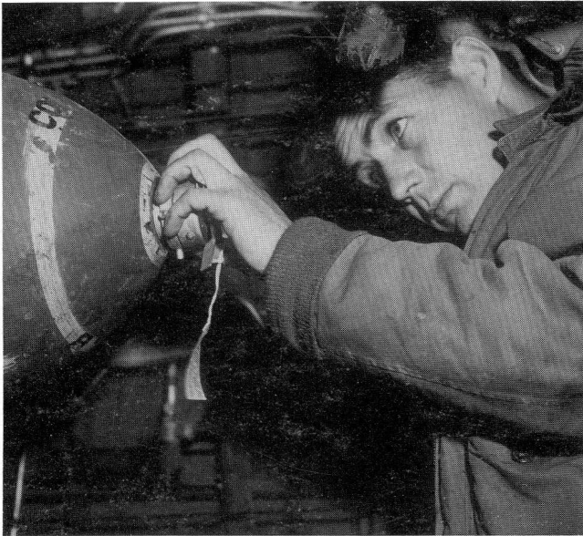
Vernell Packard 827 squadron armorer installs a nose fuse in a 500 pound general purpose bomb. 484th BG Photo via Vernell Packard
