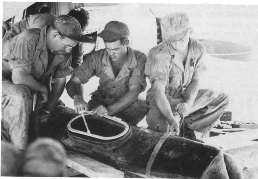
Replacing a fuel cell in Broad Abroad. From left: Cpl Art Barkley, S/Sgt Jessie Hogan, and Cpl Edgar M Livingston.
