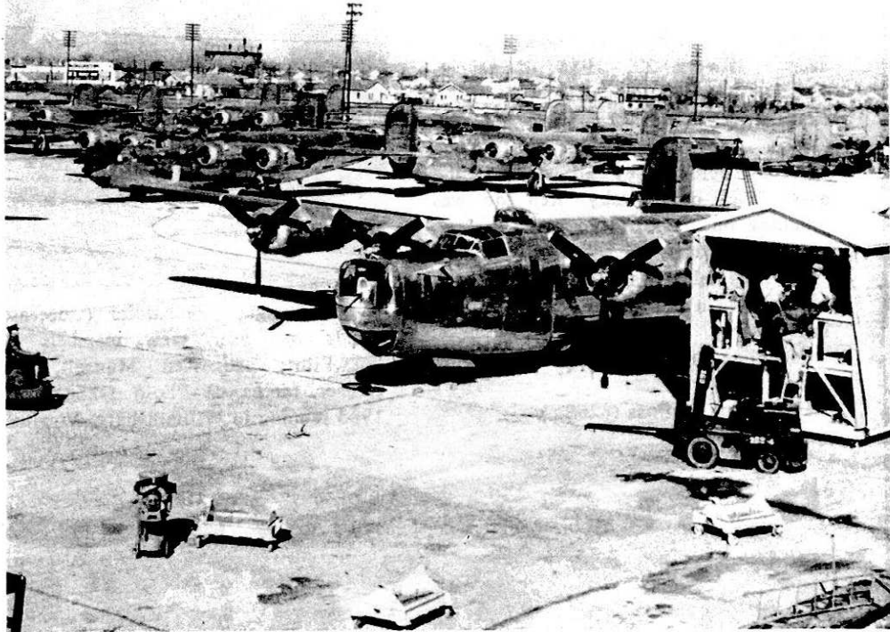
North American Aircraft production of B-24s at Dallas, Texas. Many aircraft plants located in the southwestern states often completed production work outside when weather permitted. In this photo propellers are being installed using a small hut that is moved from engine to engine as each prop is hung. This photo shows the paddle blade design propellers that replaced the slim props used on the earlier B-24D series. Bob Waag Photo.
